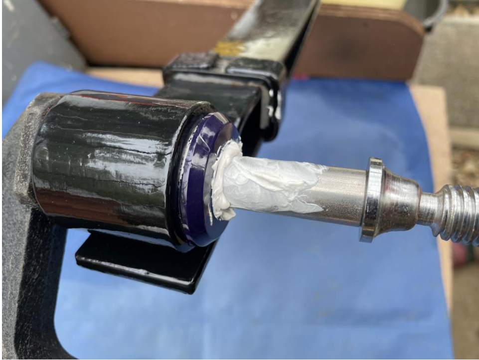
The sleeve (plus Acorn) being pressed into the bush.
